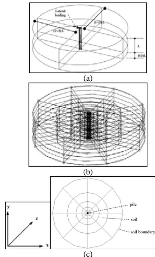
Figure 3. Details of the mesh (a) outlined (b) finite element mesh details (c) XZ plane view
