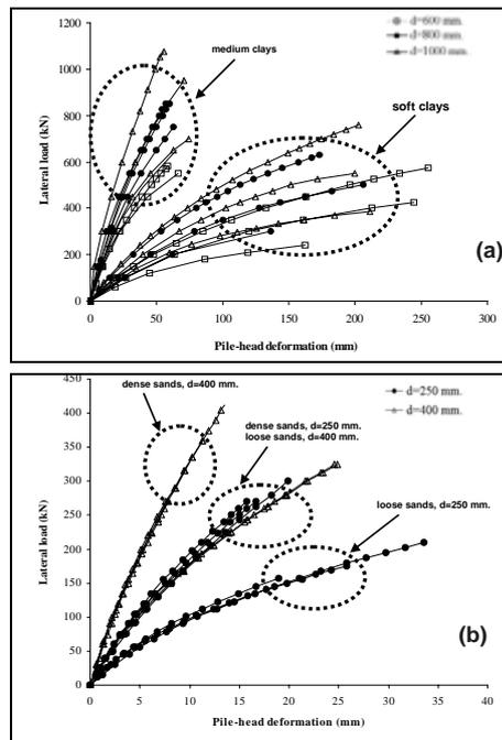
Figure 6. The pile head deformation (a) clays (b) sands
