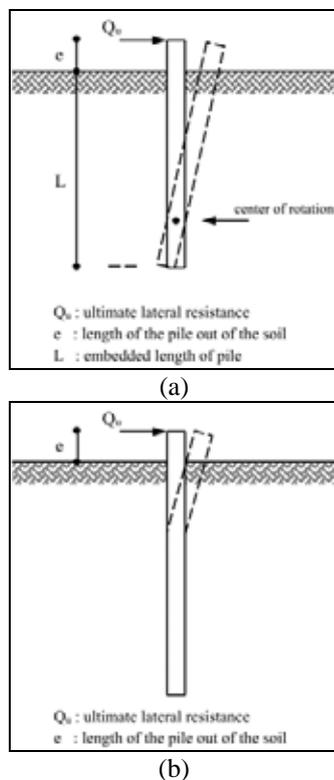
Figure 2. Deformation modes for short and long piles (a) short pile deformation (b) long pile deformation (Broms, 1964)
