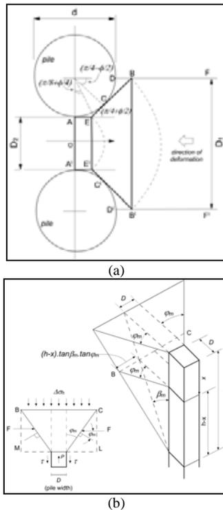
Figure 1. (a) Plastic deformation state of soil between piles (Ito and Matsui, 1975) (b) Strain wedge mechanism of soil (Ashour and Norris, 1998)
