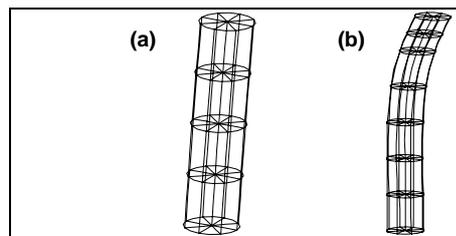
Figure 5. Pile deformation shapes from FEM (a)  $L=4$  m. short piles (b)  $L=12$  m long piles
