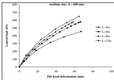
Figure 4. Load-deformation curves according to pile length of  $d=600$  mm. for medium clays
