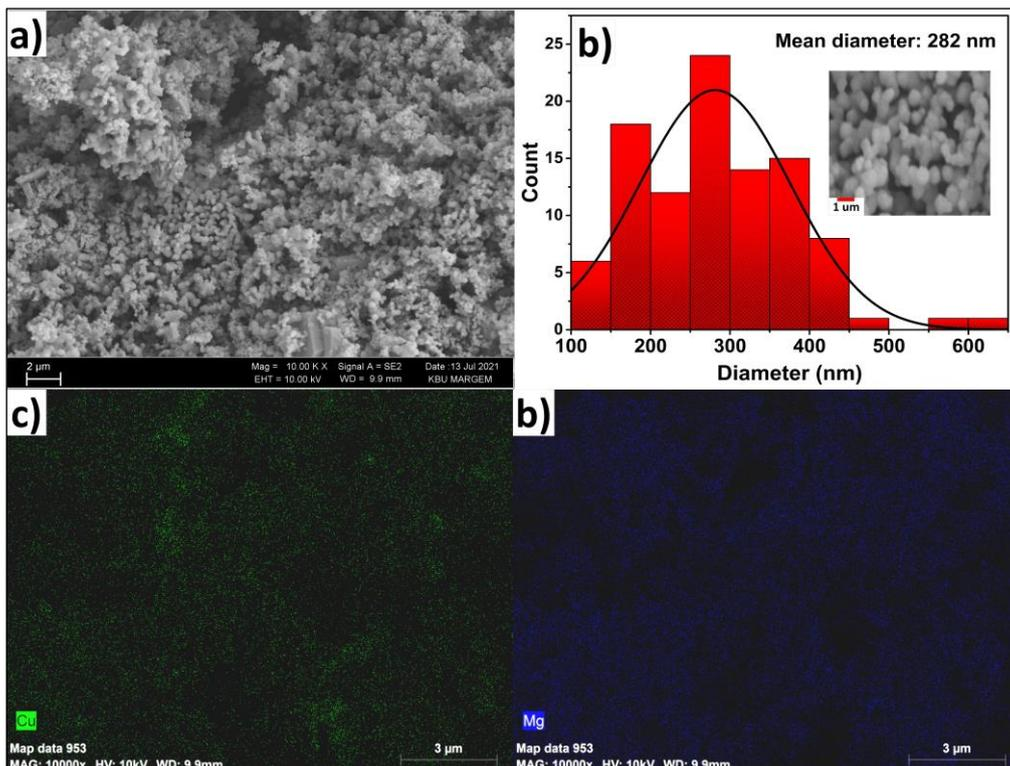
**Figure 4.** a) SEM images of MgO/CuO, b) histogram graph of particle diameter of MgO/CuO with inset images, c and d) mapping images of MgO/CuO nanoparticles
