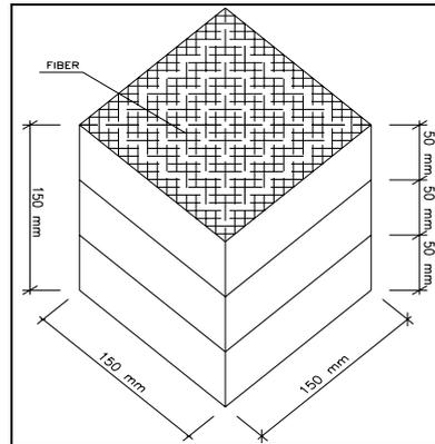
Figure 3. Shape of Samples of Mud Bricks (A3-B3-C3-D3)
