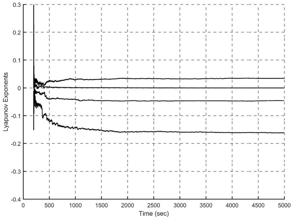
**Figure 6.** Lyapunov exponents graph of cutting process system
