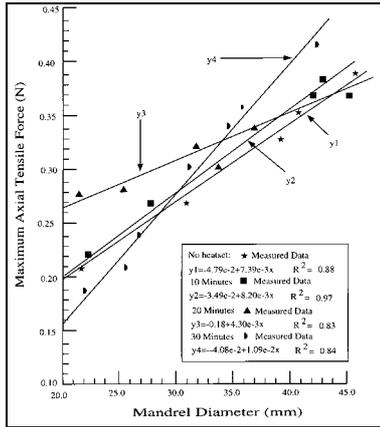
Figure 13. Effect of heat set duration on tensile force (32 yarns, heat set temperature 234 °C)
