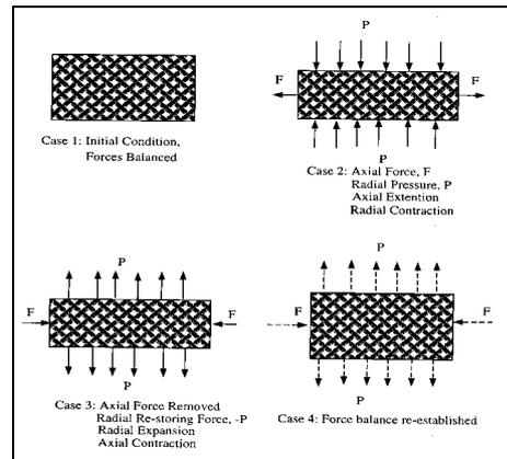
Figure 2. Structural changes in a stent under the influence of forces
