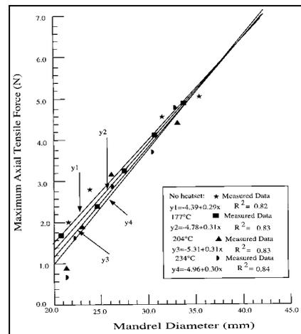
Figure 12. Effect of heat set temperature on tensile force (16 monofilaments, heat set time 30 min.)
