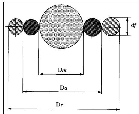
Figure 3. Cross-section of mandrel and yarn
