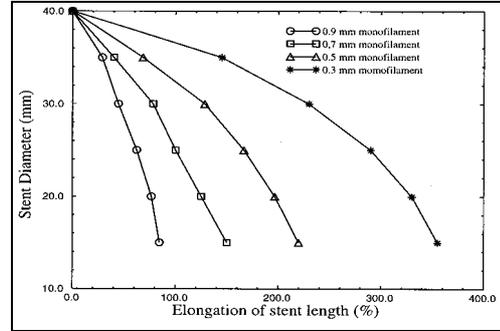
Figure 9. Variation of stent diameter with stent elongation
