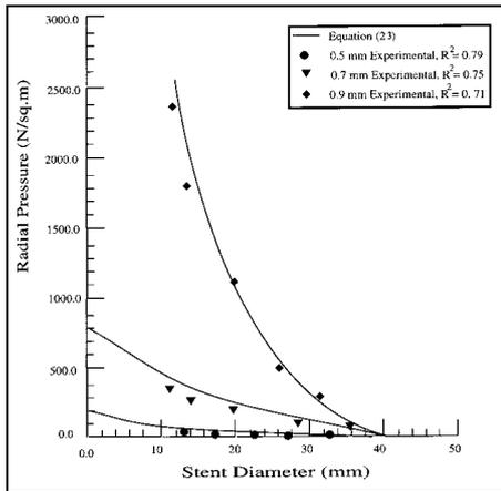
Figure 8. Theoretical and experimental radial pressure versus stent diameter for Various filament diameters
