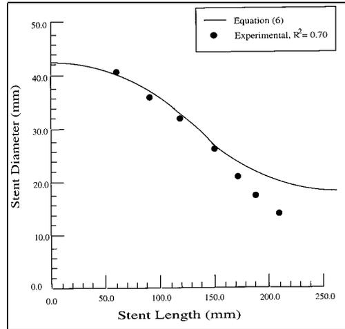
Figure 10. Comparison of theoretical and experimental data for stent length and diameter
