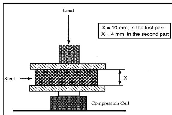
Figure 6. Schematic of compression test
