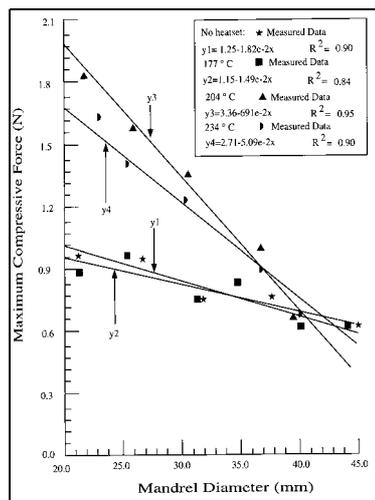
Figure 15. Effect of heat set temperature on compressive force (16 monofilaments, heat set time 30 min.)
