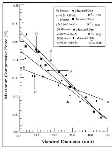
Figure 14. Effect of heat set duration on compressive force (32 yarns, heat set temperature 234 °C)
