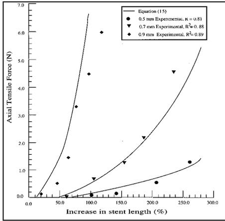
Figure 7. Theoretical and experimental axial tensile force versus stent length for various filament diameters
