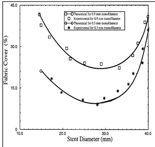
Figure 11. Effect of stent diameter on fabric cover
