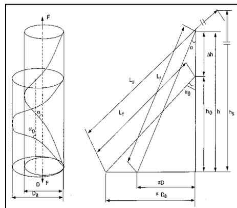
Figure 4. Geometry of braided tube before and after application of axial load
