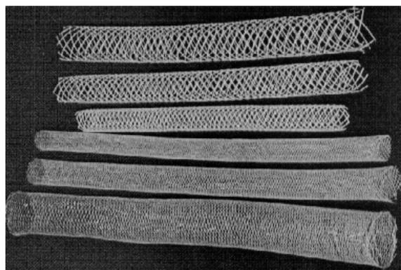
Figure 5. Some braided tubular structures manufactured for experiment
