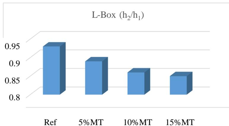
**Figure 8.** L-Box test results of SCLWC samples
