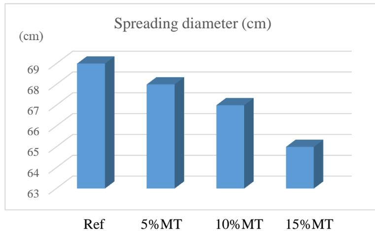
**Figure 5.** Slump-dispersion test results of SCLWC samples
