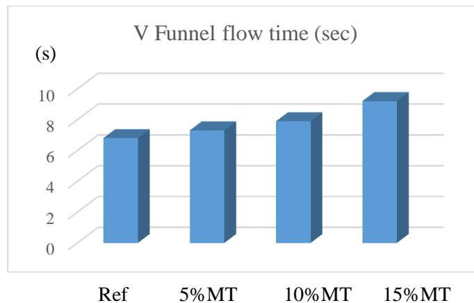
**Figure 7.** V-Funnel test results of SCLWC samples
