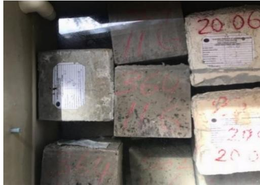
**Figure 4.** Curing of samples in curing pool
