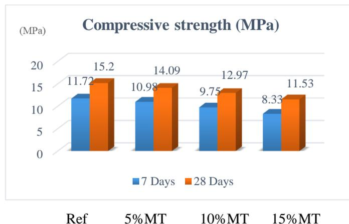
**Figure 12.** Compressive strength test results of SCLWC samples
