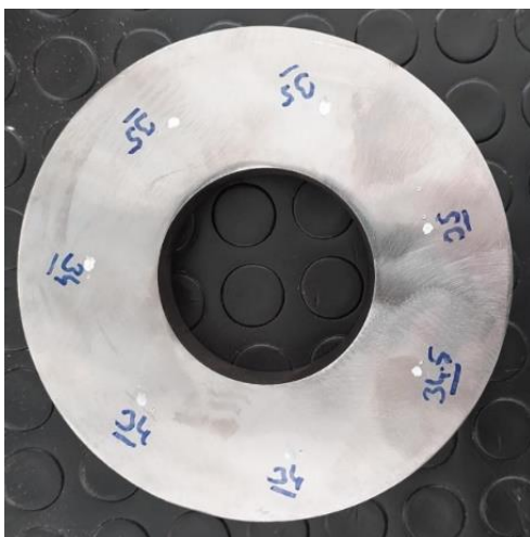
Figure 8. Hardness measurement after heat treatment
