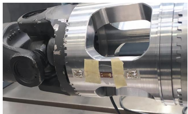
Figure 13. Strain gages dedicated for commercial board
