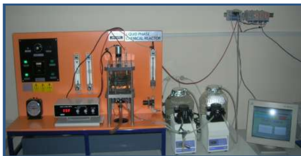
Figure 1. Experimental system for continuous saponification process
