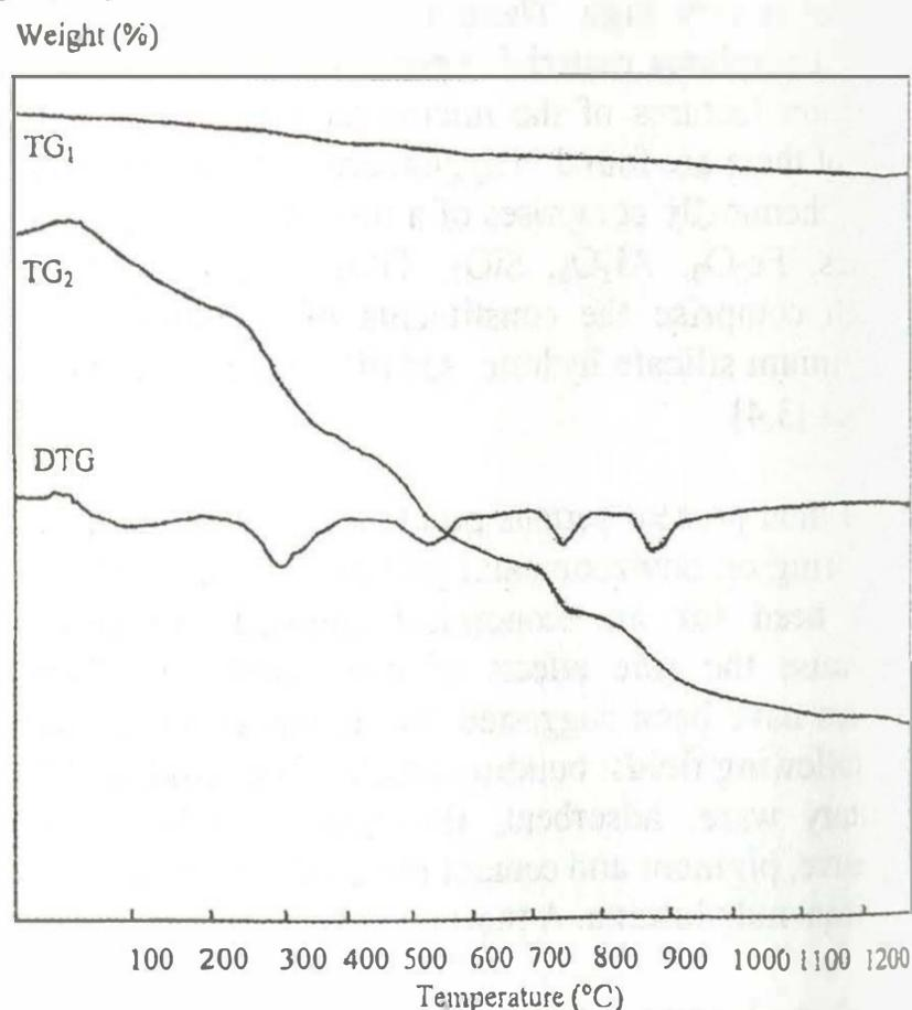
Figure 2. Thermal analysis curves of red mud
