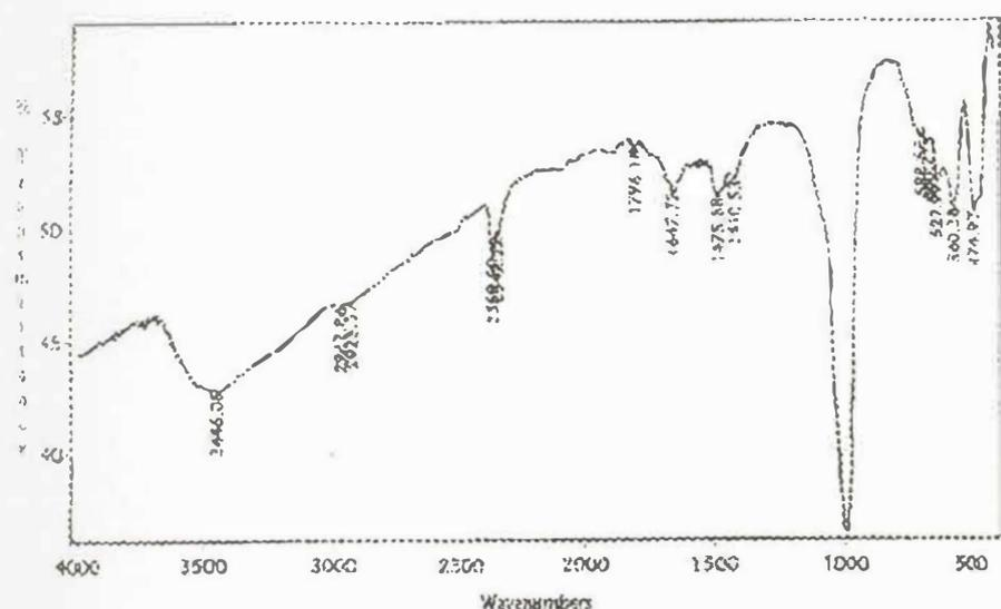
Figure 3. Infrared spectrum of red mud
