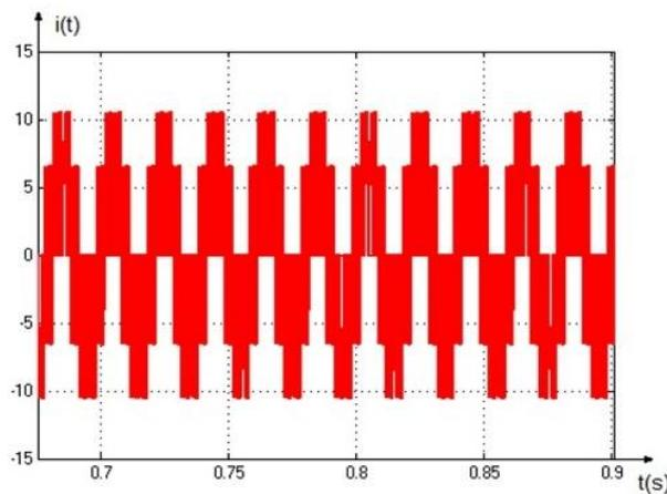
**Figure 10.** Inverter output current waveform (without filter)
