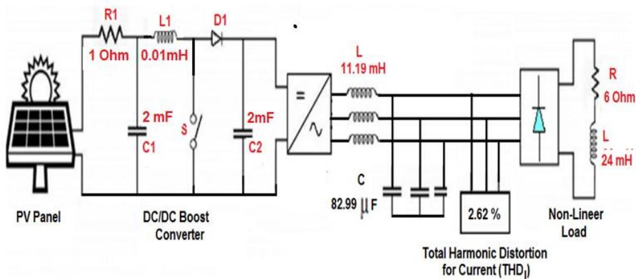
Figure 13. Off-grid PV system model with LC filter
