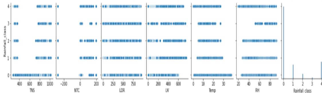
Figure 6. Relationship between sensor data and precipitation classes
