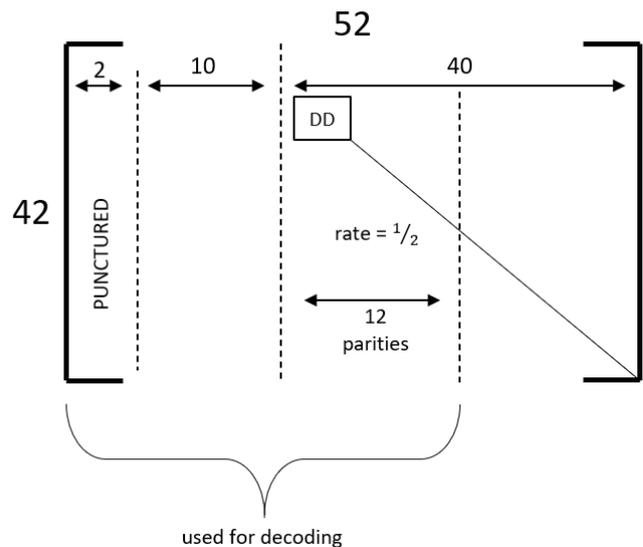
Fig. 3. LDPC, Basegraph2 – parity check matrix
