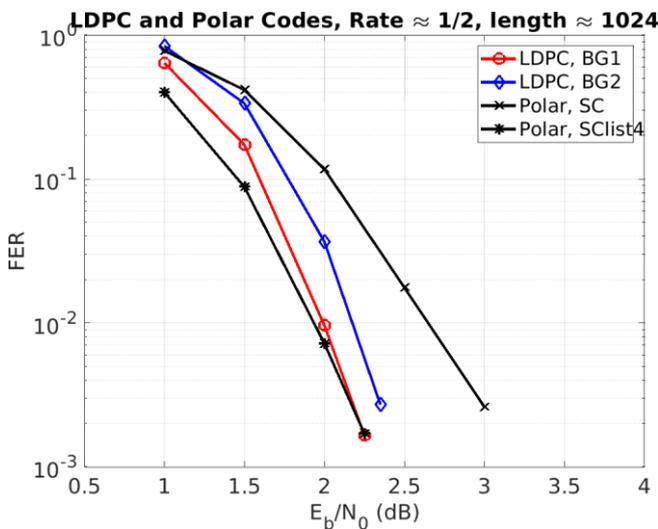
Fig. 4. LDPC and Polar Codes, Rate ≈ 1/2, length ≈ 1024
