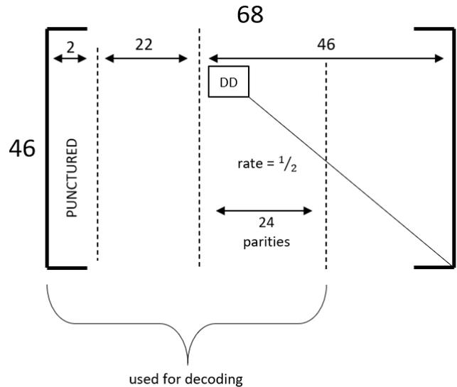
Fig. 2. LDPC, Basegraph1 – parity check matrix
