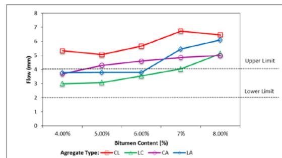
**Figure 10.** Relationship between flow and bitumen content.
