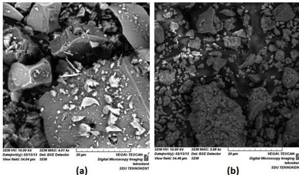
Figure 2. SEM analysis results of colemanite (a) and limestone (b) samples
