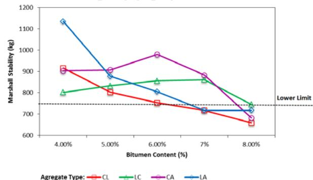
Figure 7. Relationship of stability and bitumen content
