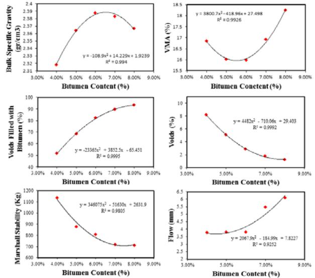
**Figure 3.** Marshall mix design values for LA
