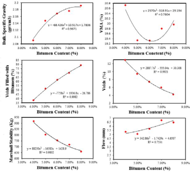
Figure 5. Marshall mix design values for CL
