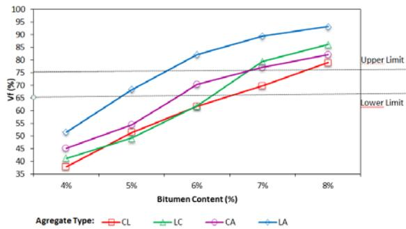
**Figure 8.** Relationship between voids filled with bitumen and bitumen content
