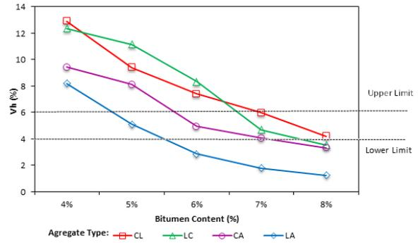
**Figure 9.** Relationship between air voids and bitumen content
