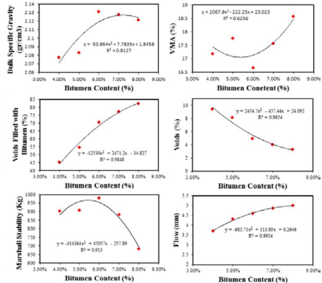
**Figure 4.** Marshall mix design values for CA
