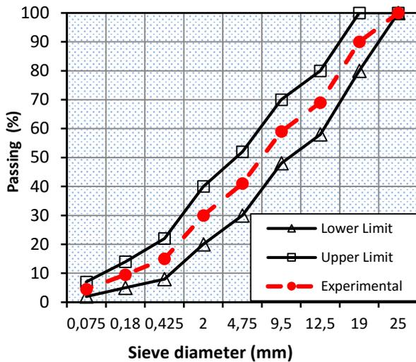
Figure 1. Gradation curve of the aggregates used in mixture
