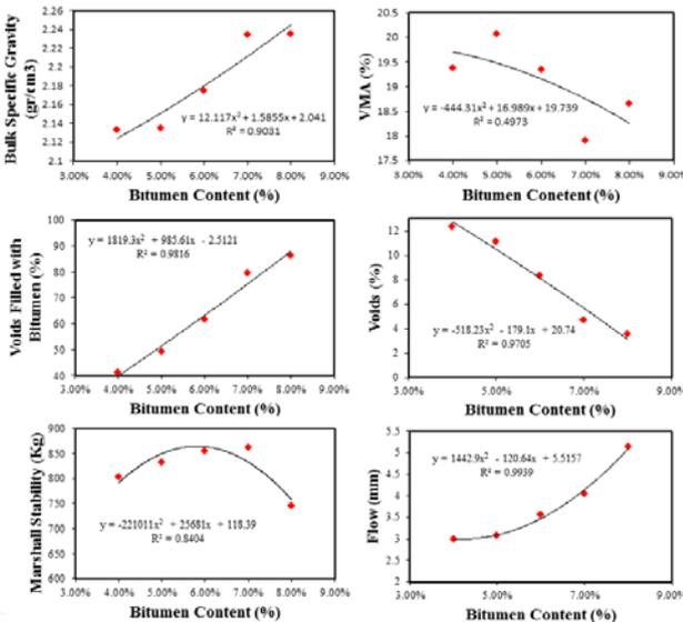
Figure 6. Marshall mix design values for LC
