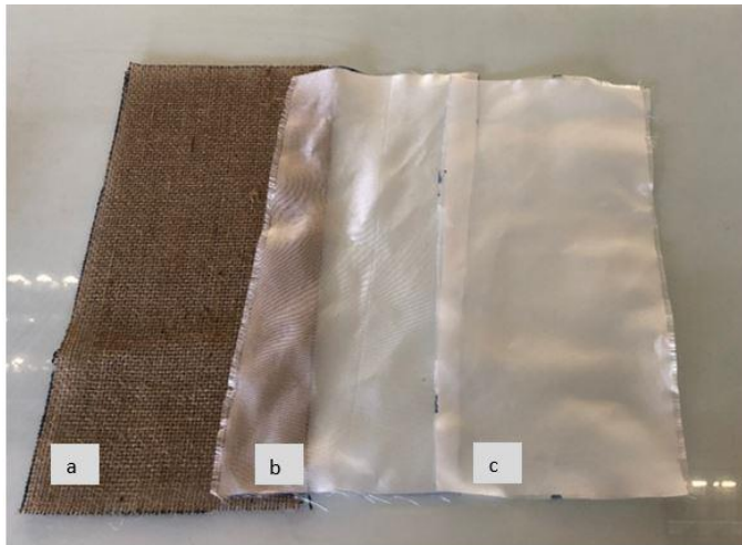
Fig. 1. Fabric samples: a) Jute b) Glass fiber (49 gr/m 2 ) c) Glass fiber (100 gr/m 2 )
