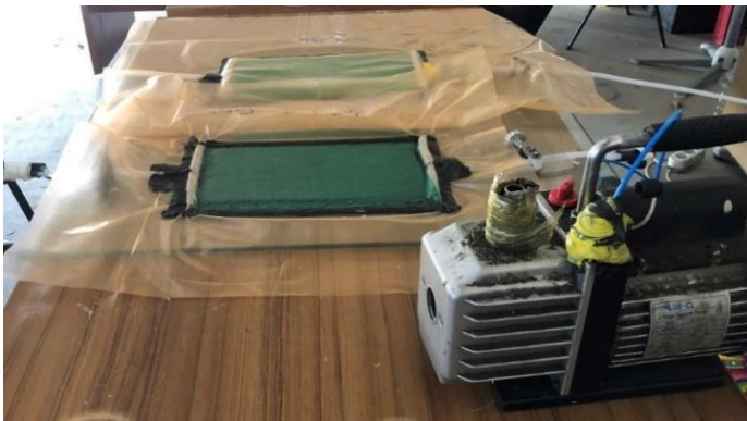
Fig. 3. Vacuum assisted resin transfer method
