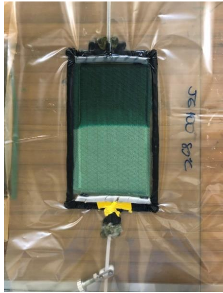
Fig. 4. Resin infusion process in Vacuum assisted resin transfer method
