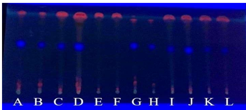
Figure 2. TLC plate under UV 366 nm, using Hexane/ EtOAc as eluent
