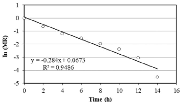
**Figure 10.** ln (MR) versus freeze-drying time for rosehip samples
