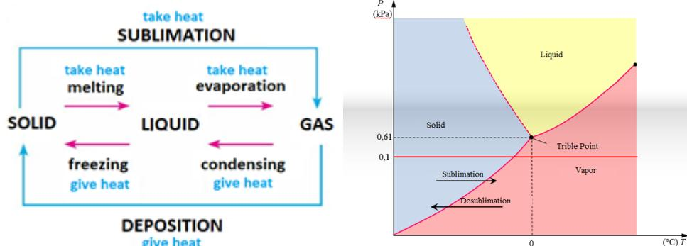
**Figure 1.** The logic of freeze-drying
