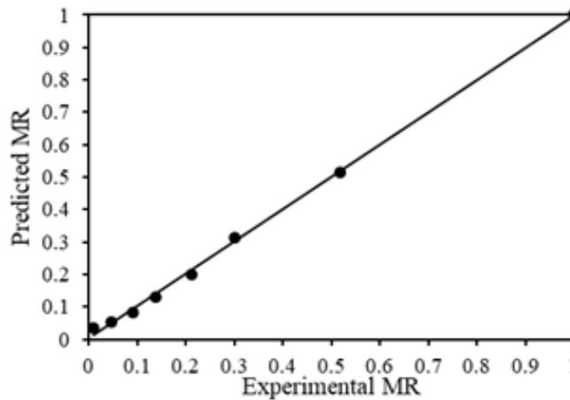
**Figure 9.** Comparison between experimental and predicted moisture ratio values applying the Diffusion Approach.
