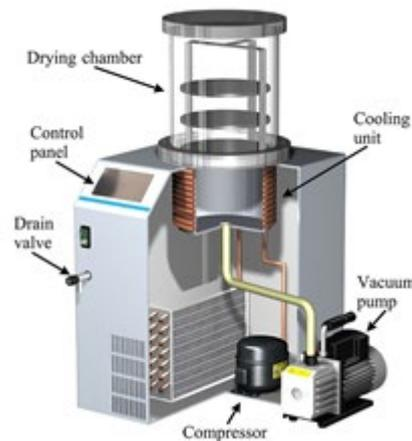
**Figure 3.** Schematic view of the freeze-drying device (Dagdeviren et al. 2021)
