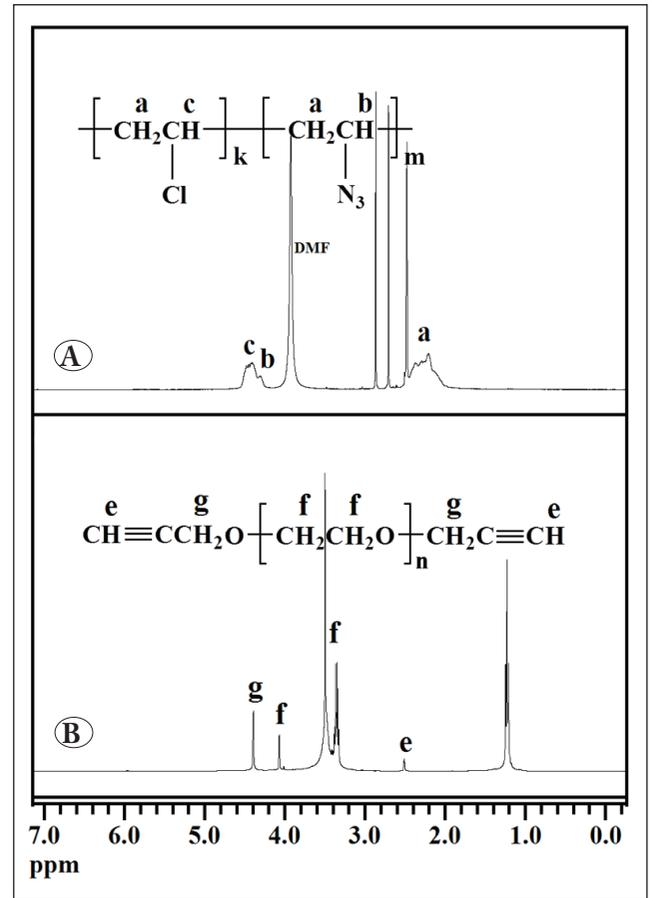
**Figure 2.** <sup>1</sup>H-NMR spectra of (A) PVC-N<sub>3</sub> and (B) dp-PEG (HH-3 in Table 1).
