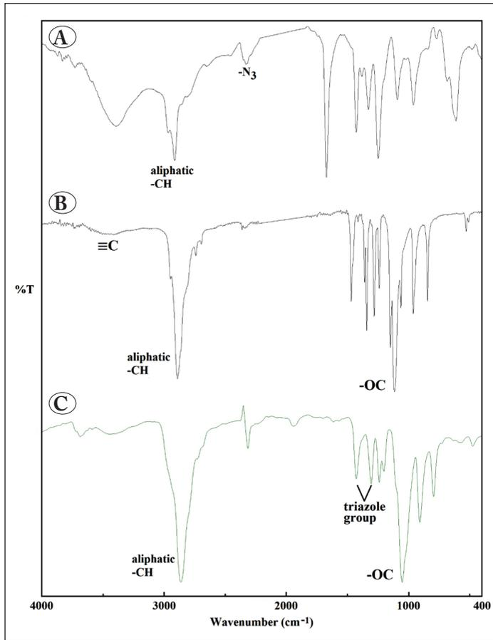
**Figure 1.** FT-IR spectra of (A) PVC-N<sub>3</sub>, (B) dp-PEG (HH-7 in Table 1), and (C) c-PVC (HK7 in Table 2).
