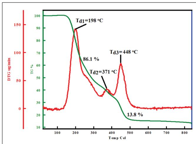
**Figure 4.** TGA thermogram of c-PVC (HK4 in Table 2).
