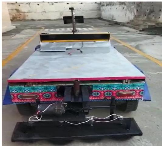
Fig. 4. The developed road cleaner
