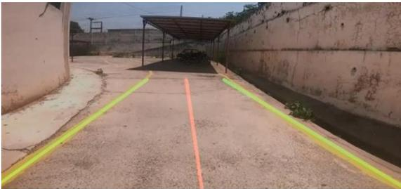
Fig. 2. Cleaner's field of view extracted lanes and heading as suggested by the algorithm
