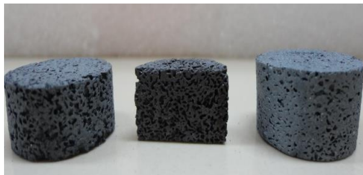
Figure 1. Photograph of the metal foams (Beköz, 2011)
