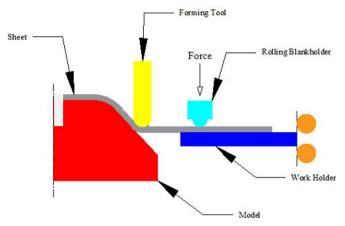
Fig. 1. Rolling blank holder method (TPIF-RL method) [10].
