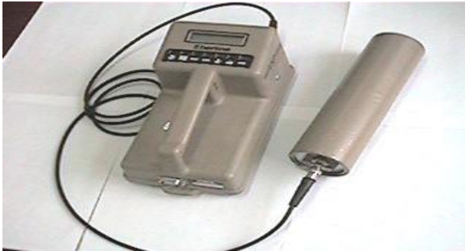
Figure 3. ESP-2 Rate meter and SPA-6 scintillation detector, Eberline [5]
