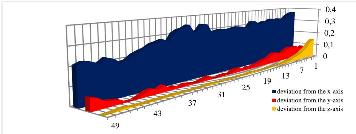
Figure 11. Deviations of the drone from the x, y and z axis during 50 seconds
