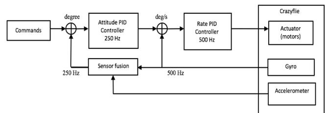
Figure 1. On-board control architecture, image courtesy of Bitcraze.
