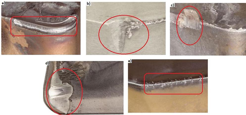
Figure 1. Wear mechanisms on the CT, a) Flank wear, b) Notch wear, c) BUE, d) Crater wear and e) Thermal crack [18]
