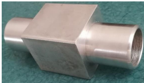
Figure 2. The aluminum device for connecting the TEG
