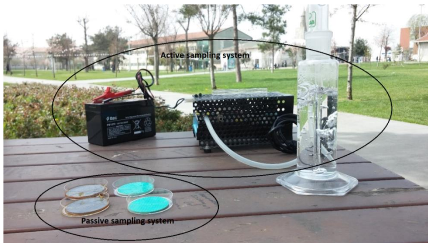
Figure 1. Active and passive sampling systems.
