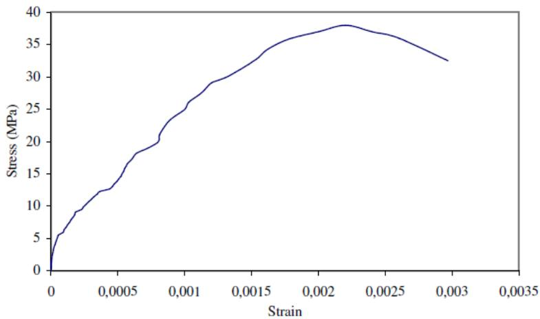
**Figure 10.** Stress-strain curve for ordinary (0.50% fiber) concrete
