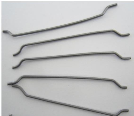
Figure 6. Steel fibers
