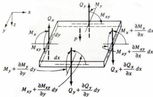
**Figure 1.** Internal forces generated within a plate [1,2]
