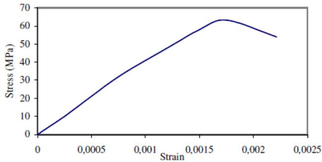
**Figure 9.** Stress-strain curve for high-strength (1.0% fiber) concrete
