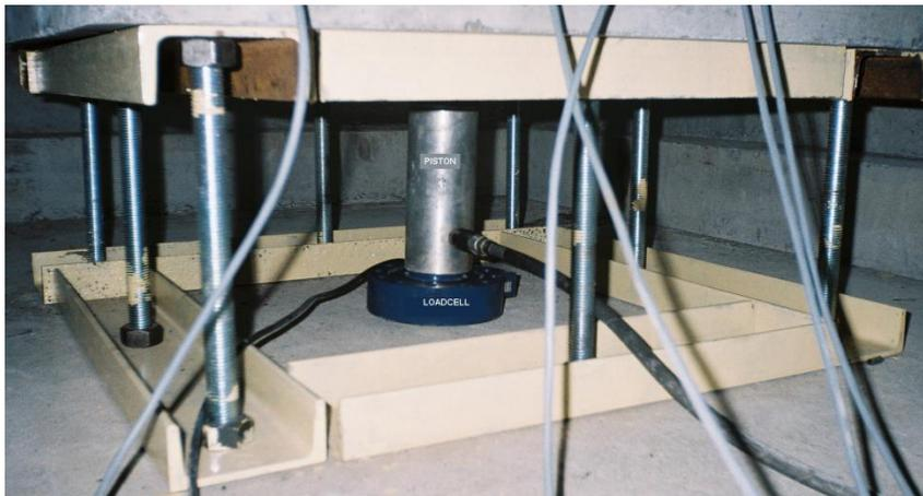
**Figure 2.** Loading piston and load-cell
