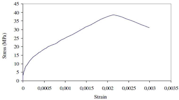
**Figure 11.** Stress-strain curve for ordinary (1.0% fiber) concrete
