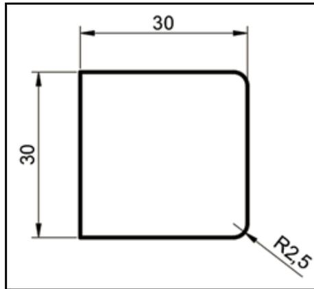
**Figure 1.** Dimensions and geometry of the samples to be cut
