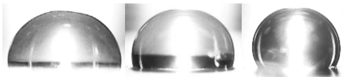
Figure 1. The contact angles of liquid droplets on the hydrophobic surfaces.
