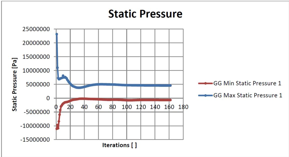
**Figure 15.** Pressure change of propeller turbulator over time
