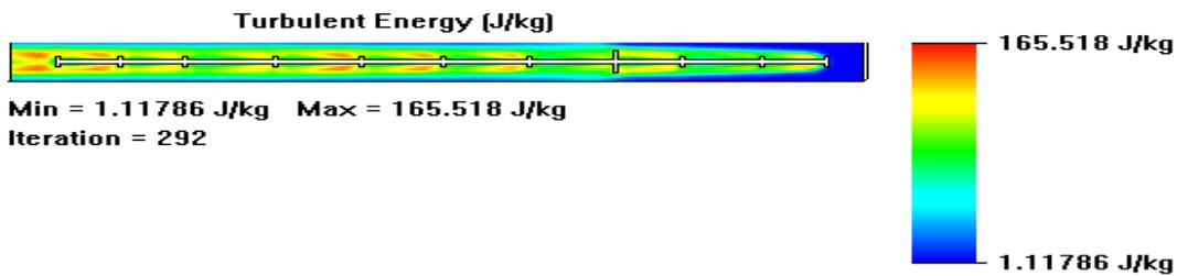
**Figure 21.** Propeller turbulator turbulence energy exchange
