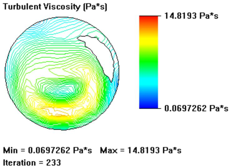
**Figure 24.** Spring turbulator turbulence viscosity change analysis
