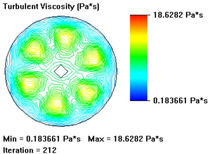
**Figure 25.** Propeller turbulator turbulence viscosity change analysis
