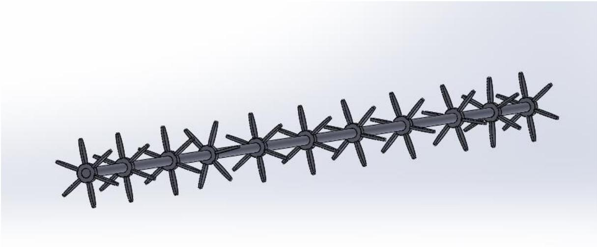
**Figure 5.** Solid model of propeller type turbulator
