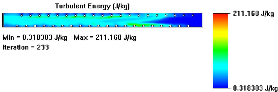
**Figure 20.** Spring turbulator turbulence energy change
