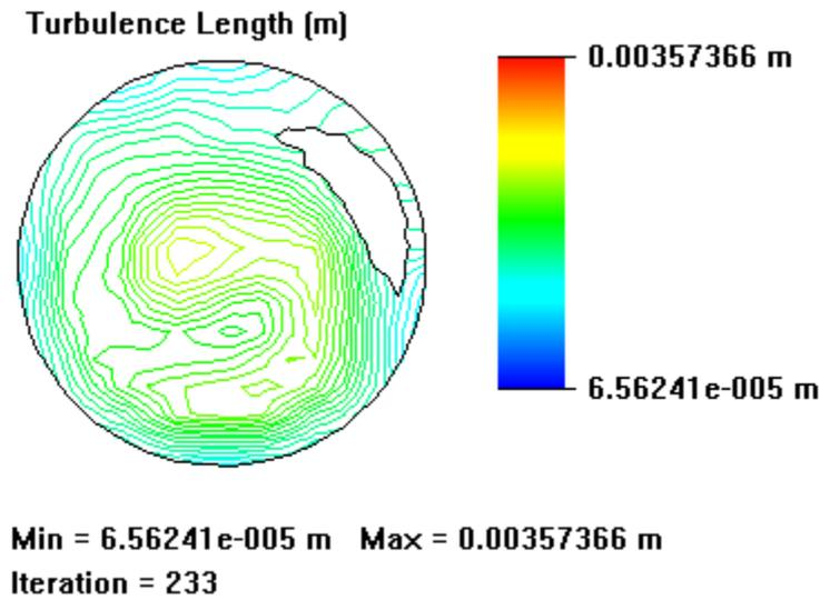
**Figure 28.** Spring turbulator turbulence length change analysis
