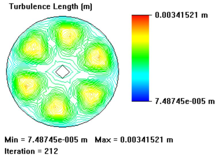
**Figure 29.** Propeller turbulator turbulence length change analysis
