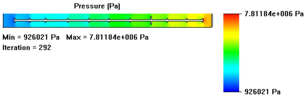
**Figure 13.** Propeller turbulator pressure change
