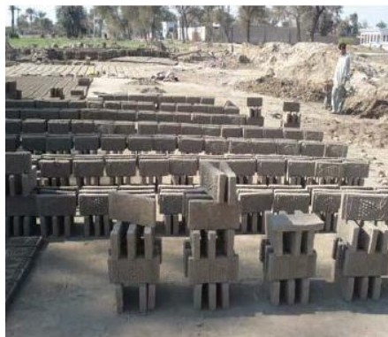
Figure 1. Sun drying processes of brick [11]
