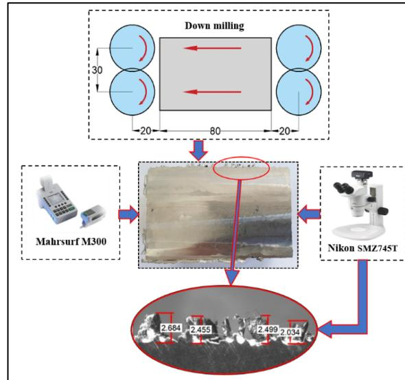
Figure 2. Measurement of Ra and burr height
