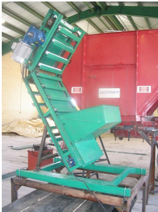
Figure 4. Fabricated metering device positioned on test rig
