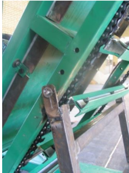
Figure 5. Adjustment arm for upper chassis angle adjustment
