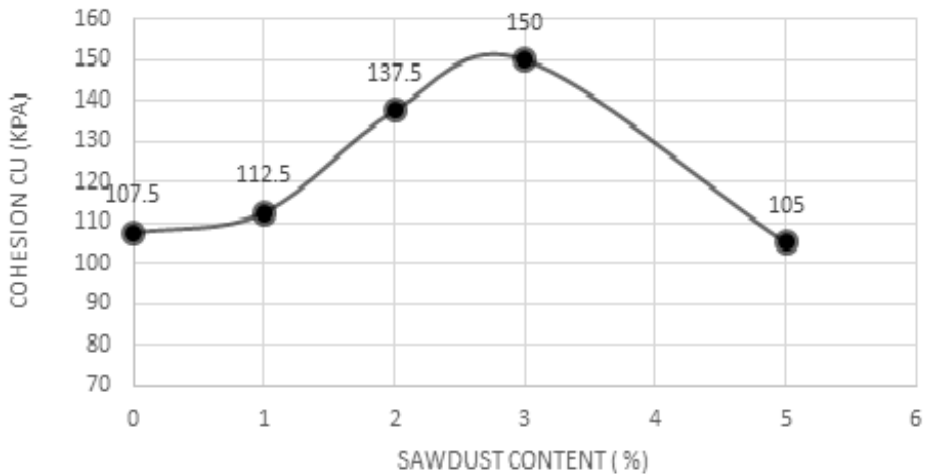
Figure 8. Effect of Sawdust on the Cohesion of the soil in the Unconsolidated Undrained Triaxial Test.
