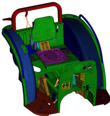
Figure 6. FE Mesh Model for Platform Structure
