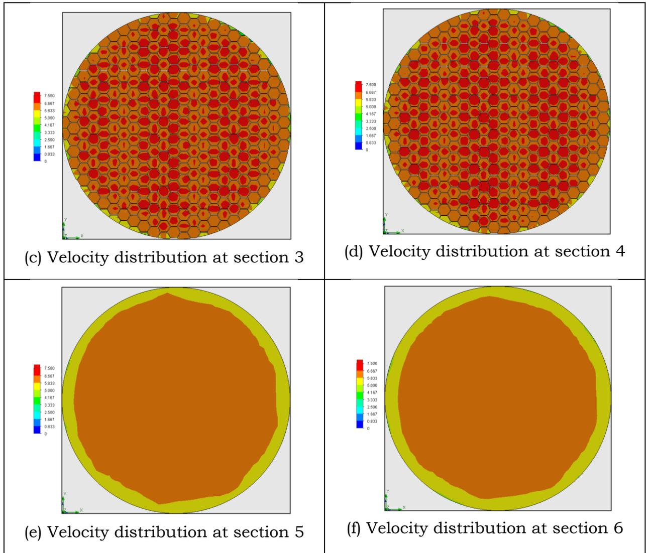
**Figure 7.** Velocity distribution of hexagonal honeycomb
