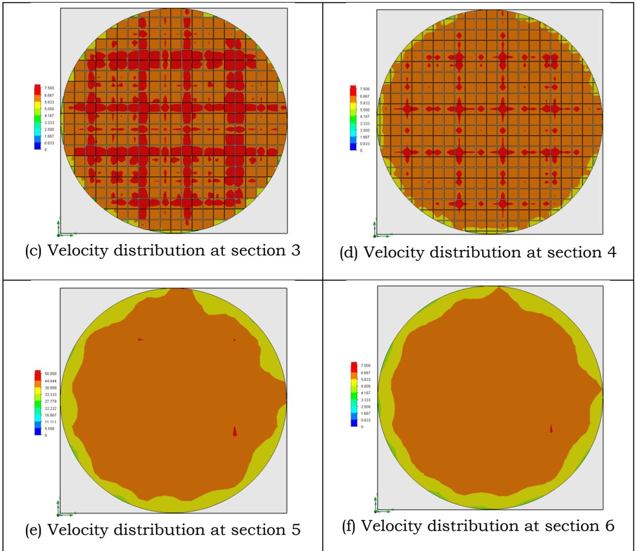
**Figure 8.** Velocity distribution of square honeycomb
