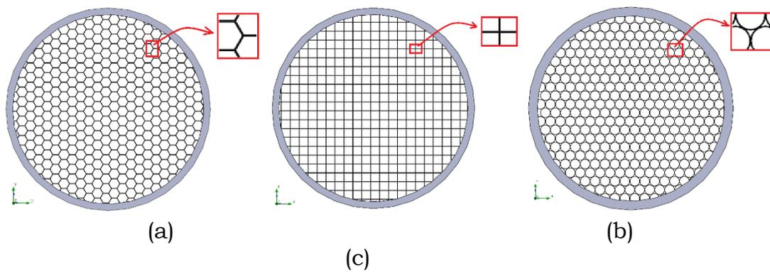
**Figure 1.** (a) hexagonal, (b) square, and (c) circular sectioned honeycomb models
