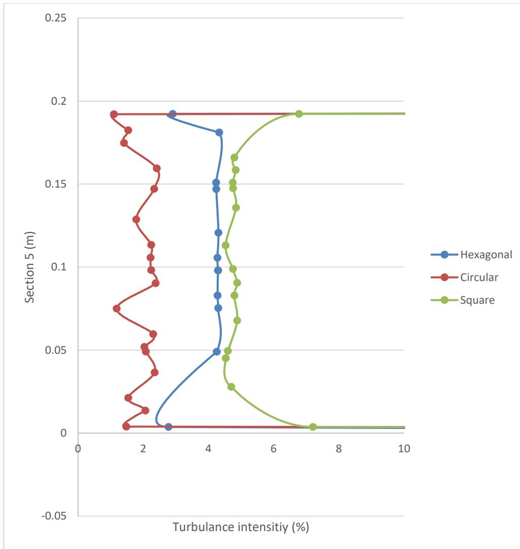
**Figure 11.** Turbulence intensity values at section 5
