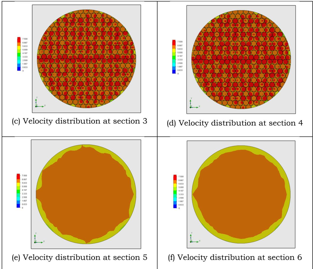
**Figure 9.** Velocity distribution of circular honeycomb
