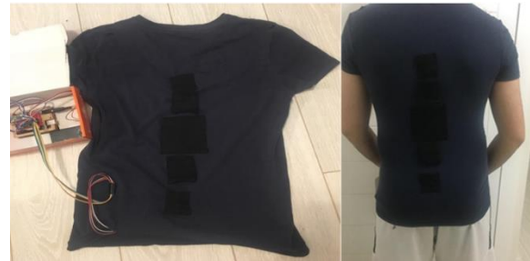
Figure 3. First prototype of posture monitoring vest with multiple pockets on the back to place accelerometer sensors.
