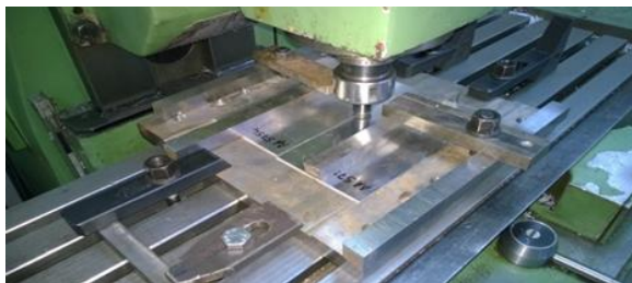
Fig 2.5 The milling machine used for friction stir welding process. Welding is performed with fixed clamping shoe parts.
