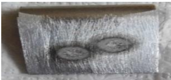
Fig 2.2 Determination of the chemical analysis by the spectral analyzer of the aluminum material used in the welding process.
