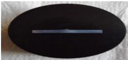
Fig 2.11. Mounting friction stir welded sample was obtained and cross-sectional sample of Mountains.
