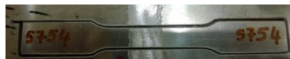
Fig 2.8 Front view of the water jet cutting part of the extrusion according to the ASTM standard test sample of the welded sheet [13].
