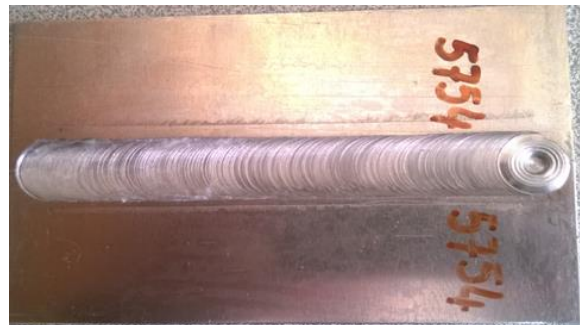
Fig 2.6 With friction stir welding method macrograph of accurate combined AA 5754 aluminum alloy sheet
