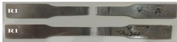
Fig 2.19 Tensile specimen after fracture; the FSW accomplished at tool rotational velocity of 1600 rpm, tool traverse speed of 125 mm/min (ASTM E8M-04).
