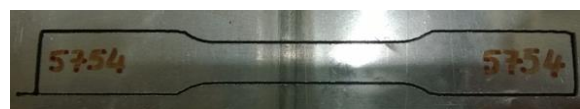
Fig 2.9 Reverse view of the water jet cutting part of the extrusion according to the ASTM standard test sample of the welded sheet [13].
