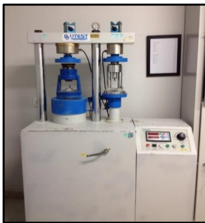
Figure 7. Compressive and splitting tensile strength equipment
