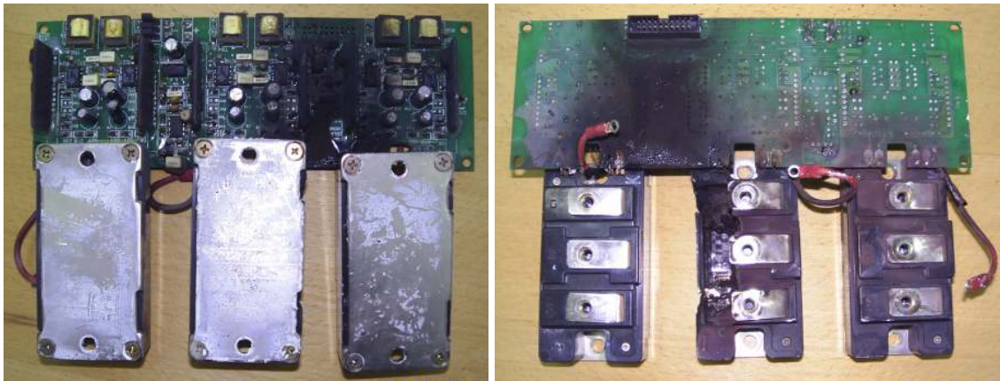
Figure 5. Front and back view of the failed card and IGBTs
