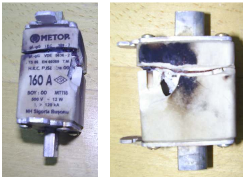
Figure 6. Front and back view of the broken rectifier circuit fuse
