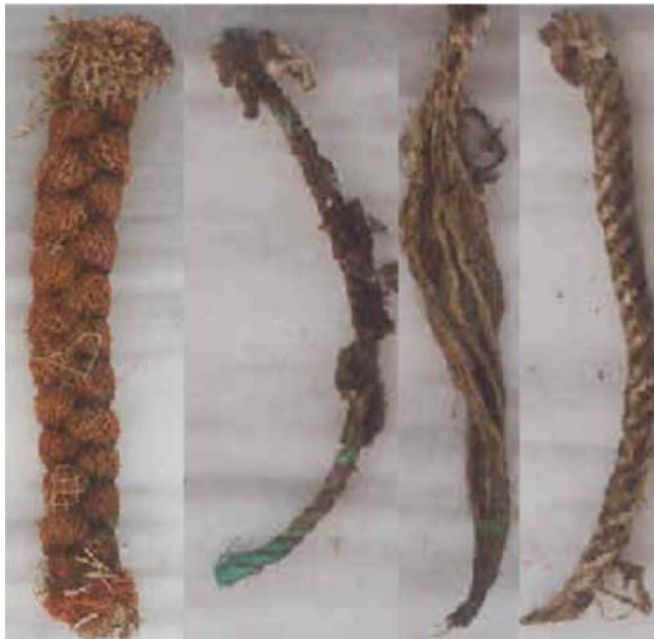
Figure 4. Collectors types (respectively, net rope, polypropylene rope, sisal rope, and jute rope) appearance after 3 months.
