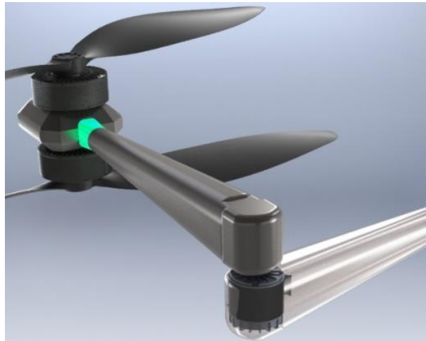
Figure 4: Designed rotor arm system
