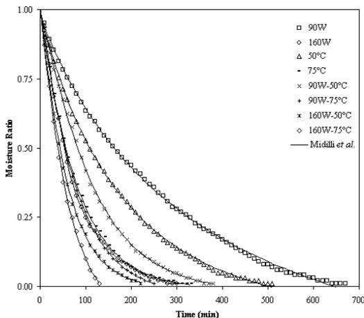
**Figure 2.** Variation of experimental and predicted moisture ratio by the Midilli *et al.* model with drying time at different drying conditions
