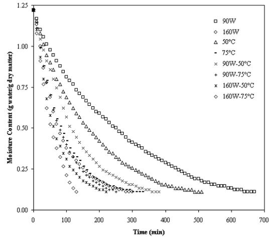
**Figure 1.** Drying curves of barbania samples at different drying condition
