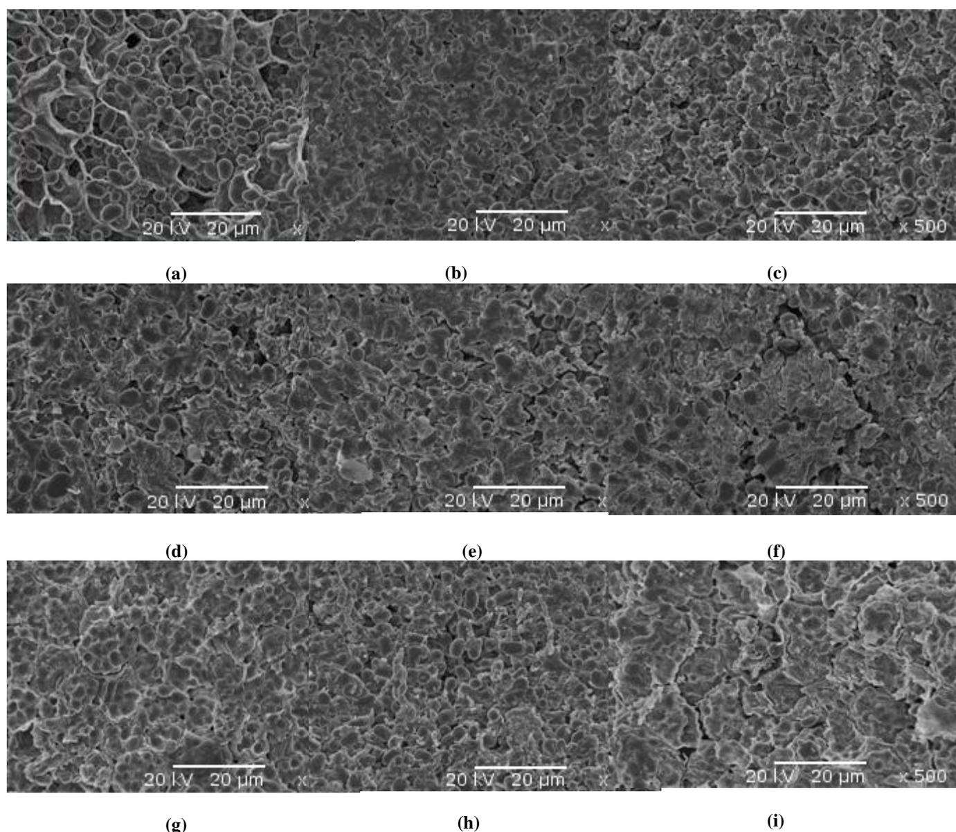
**Figure 3.** SEM images of fresh and dried barbania beans: fresh (a), microwave drying at 90W (b) and 160W (c), convective drying at 50°C (d) and 75°C (e), microwave-convective drying at 90W-50°C (f), 90W-75°C (g), 160W-50°C (h) and 160W-75°C (i)
