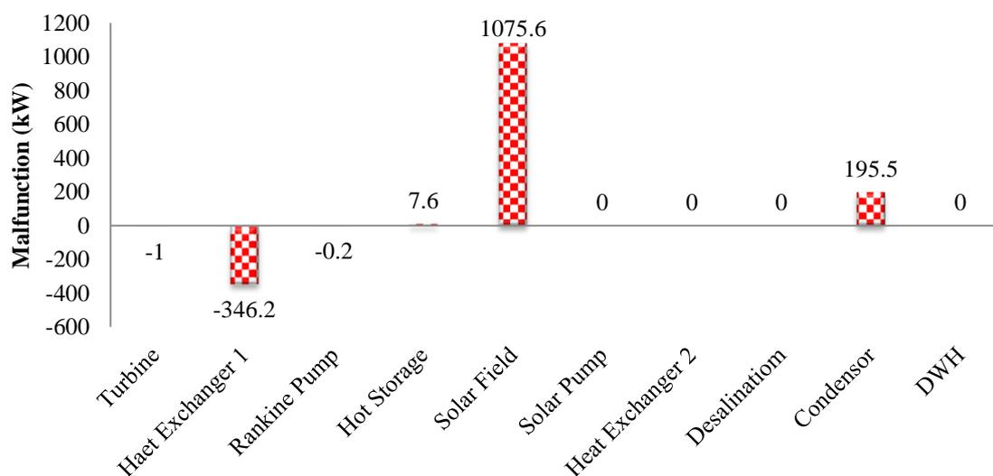
Figure 3. The different components Malfunction of the proposed cycle
