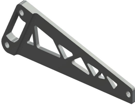
Figure 7. The revised solid model of the load-carrying element after the optimization process
