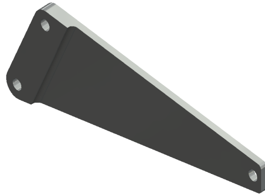
Figure 2. The solid model of the load-carrying element
