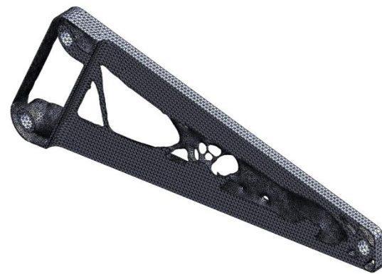
Figure 5. The non-parametric void model after the optimization process
