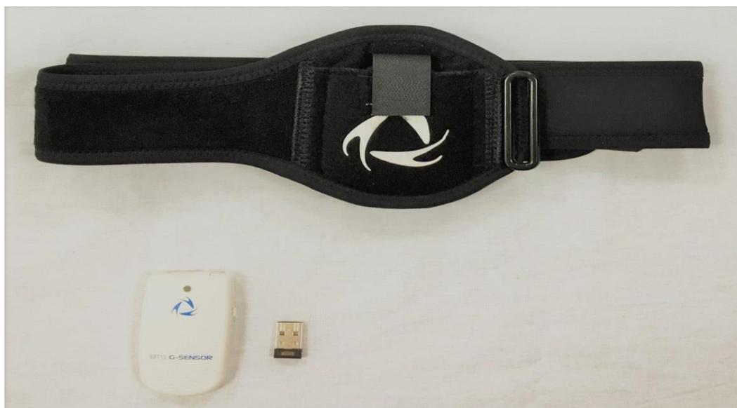
**Figure 1:** BTS G-WALK Tempora-Spatial wireless digital gait analysis system
