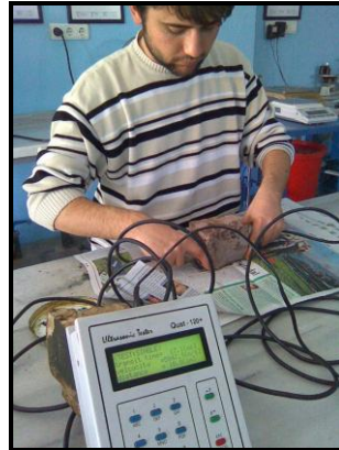
Figure 2. Ultrasonic pulse velocity measurement
