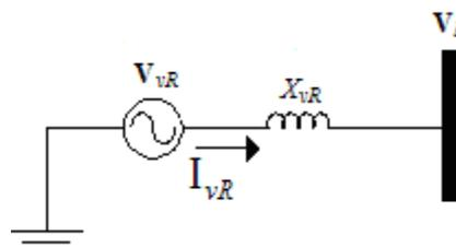
**Figure 2.** STATCOM equivalent circuit
