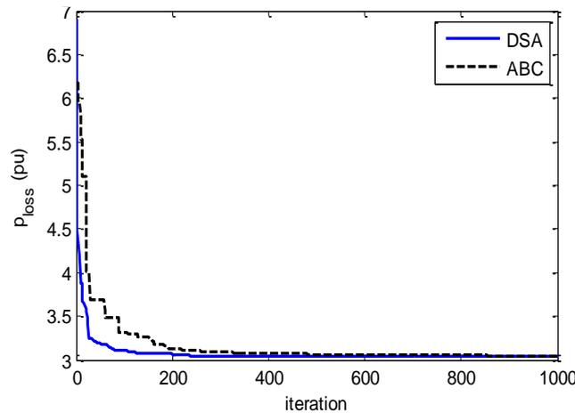
**Figure 4.** Convergence curves of two optimization algorithm for minimizing active power loss
