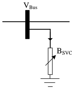
**Figure 1.** Susceptance model of SVC
