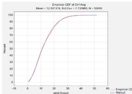
**Figure 7:** Weibull Distribution Fit for the Biga Site Wind Speed Data
