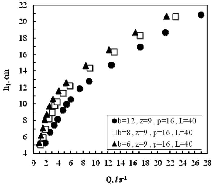
Figure 5-Head-discharge curves for various crest width ( $b$ )
