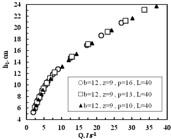
**Figure 4-Head-discharge curves for various weir height ( $P$ )**
