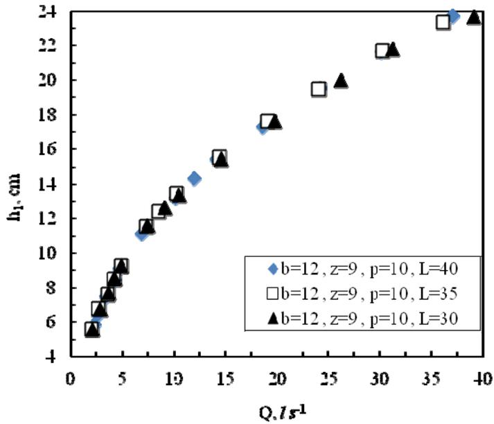
Figure 6-Head-discharge curves for various crest length ( $L$ )
