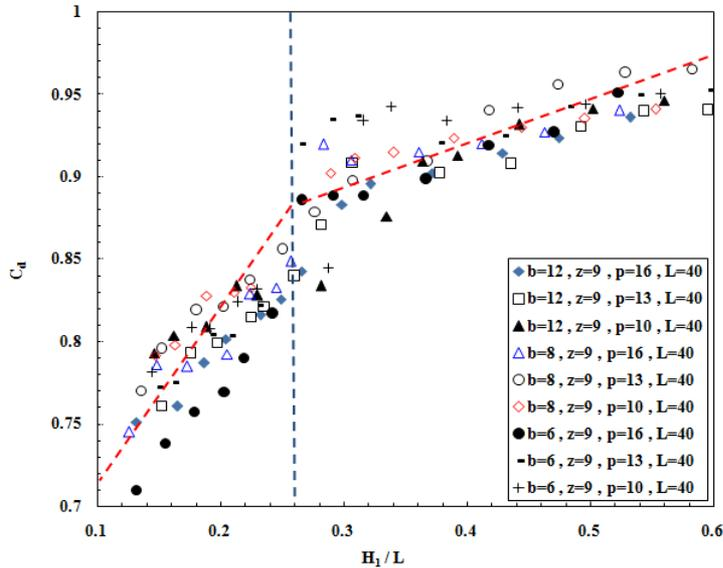
**Figure 7-**  $C_d$  versus  $H_1/L$  for varying  $P$  and  $b$  and constant  $z$  and ( $L$ )
