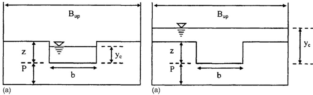
**Figure 3**-Two different flow cases through weir section: (a) Case 1; (b) Case 2
