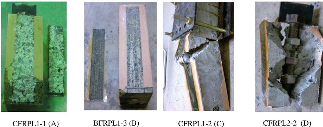
**Figure 3:** Typical failure mode of FRP specimens
