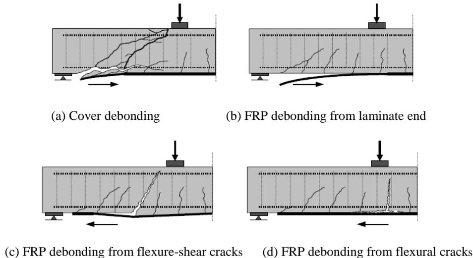
**Figure 1:** Debonding failure mechanism of FRP strengthened beams
