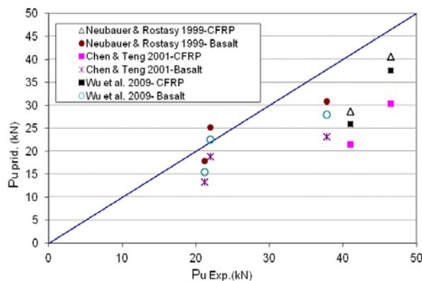
**Figure 2:**  $P_u$  predicted versus  $P_u$  experiment for different types of FRP composites using Flexible adhesive layer
