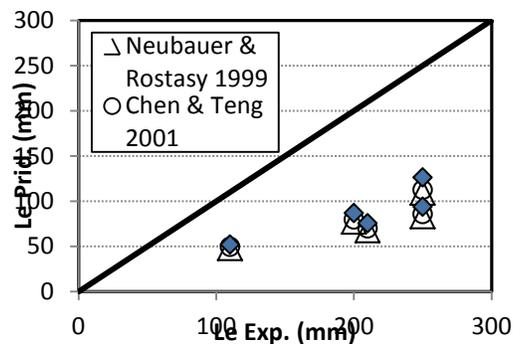
**Figure 4:**  $L_e$  predicted versus  $L_e$  experiment for different types of FRP composites using Flexible adhesive layer
